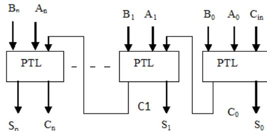
**Figure.2** Design of n-bit PASTA using Mux
